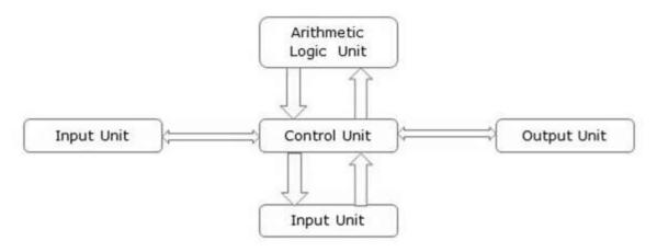
The basic parts of a computer are as follows –
